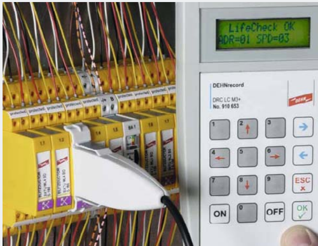
Testing an SPD module via RFID technology
